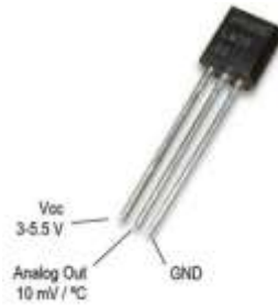
Fig. 3. Temperature Sensor (LM35)
